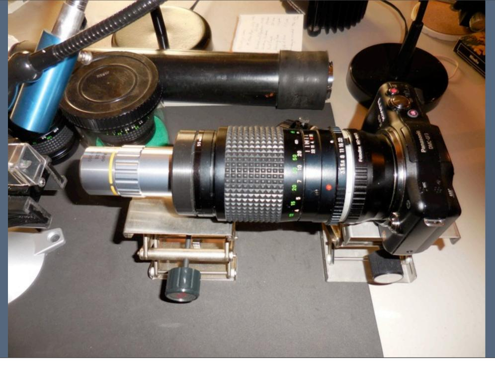
Mitutoyo Lens, adding Bellows to increase magnification
