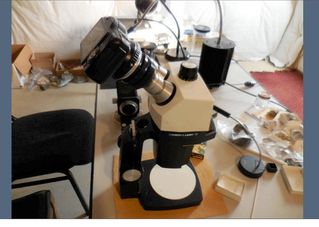
Further zooming-in using Stereo microscope, and stacking 4 images
